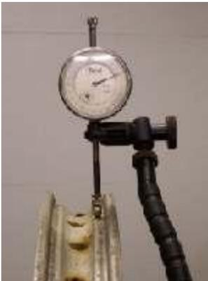
Now screw in the nipples the same amount on each spoke and finger tight. Take the assembled wheel and put it on the bike and tighten the axle. If it's a rear wheel, adjust it like you would if you were adjusting the rear chain. Now comes the fun part. Truing the wheel. You wheel must be no more than two, onehunderths of an inch in out of roundness and side play. Set up a dial micrometer to measure out of roundness and side play.
