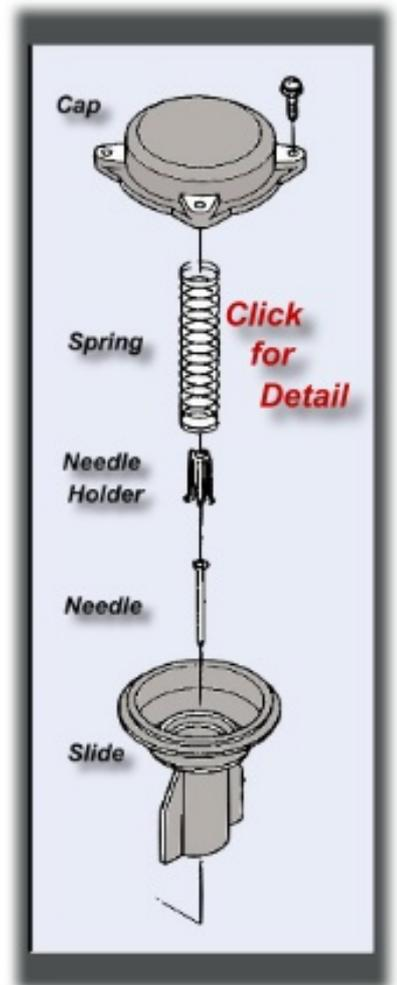
Every component deserves inspection throughout all procedures discussed. Pam Falcioni mentions: check that float valve "needle" and seat! A likely source of crummy idling, starting, etc. Anything bashed, scored, bent and so on needs repair or replacement. Common sense prevails. Do all parts function correctly, slide easily and seat tightly where they should? Make it happen!
